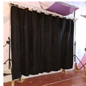
PX500 FABRIC 100% CARBON FIBER (~5 mm thick & 500 gr/m 2 )
