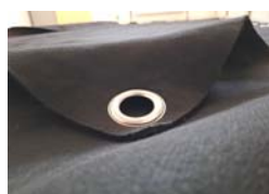
PX500 FABRIC 100% CARBON FIBER (~5 mm thick & 500 gr/m 2 )
