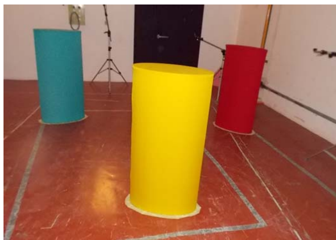
Photo of the 3 samples in reverberation room
