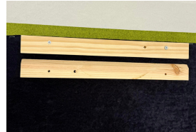
Colgado con medias maderas Hanging with two half-lap joint
