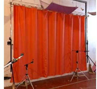
ILUCS FABRIC 100% POLYESTER TREVIRA CS (~0,5 mm thick & 265 gr/m 2 )
