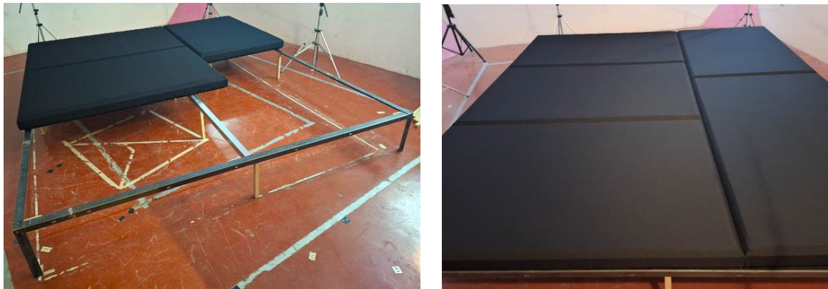
Photos of mounting of test specimen
