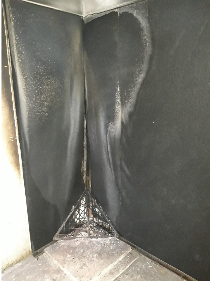
Appearance of the sample after the SBI test as per EN 13823
