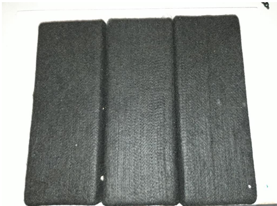
Appearance of the sample before the ignitability test according to EN ISO 11925-2 (application on surface)
