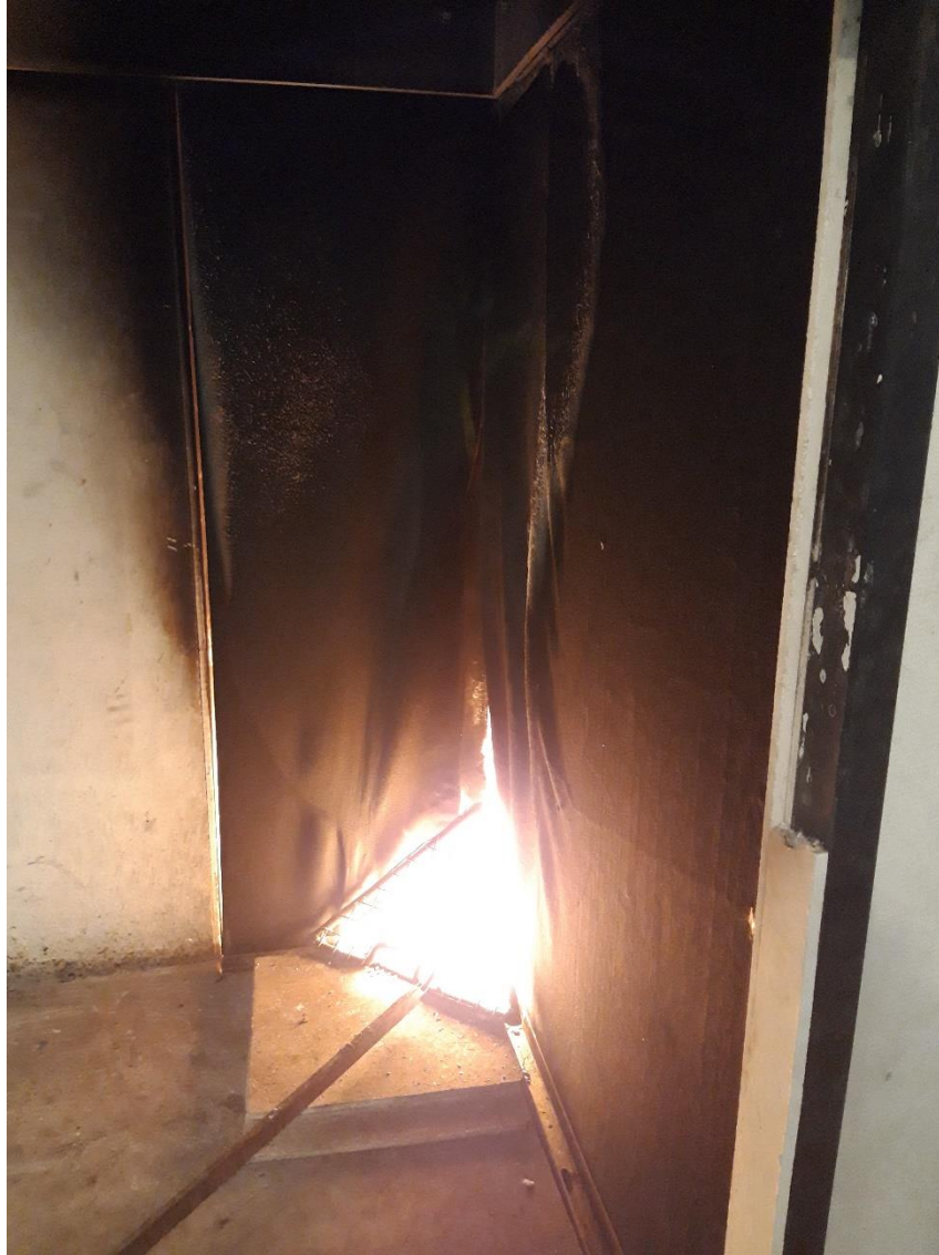
Appearance of the sample during the SBI test as per EN 13823
