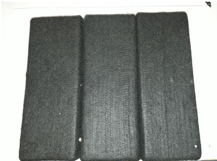
Appearance of the sample before the ignitability test according to EN ISO 11925-2 (application on edge)
