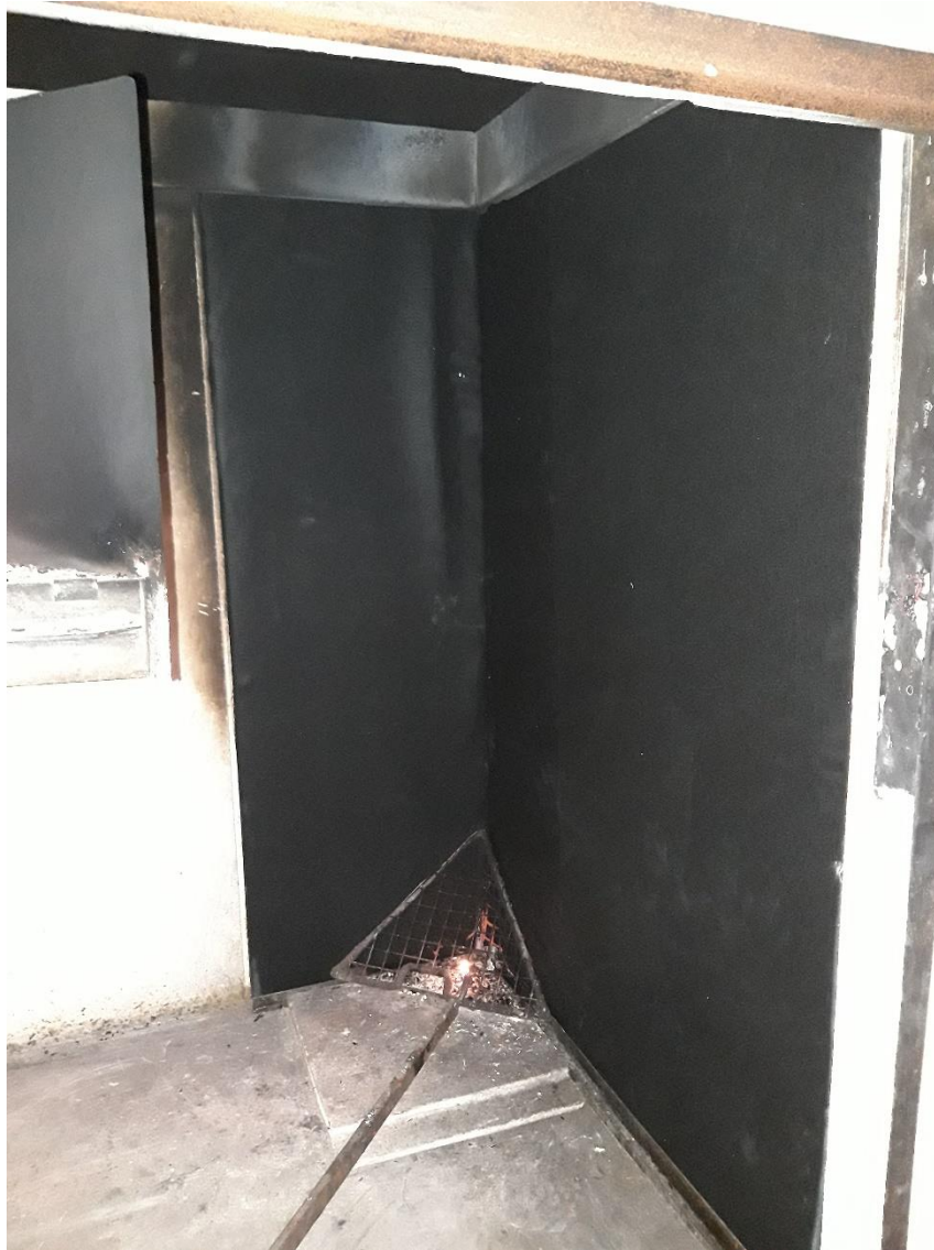
Appearance of the sample before the SBI test (short wing and long wing) as per EN 13823
